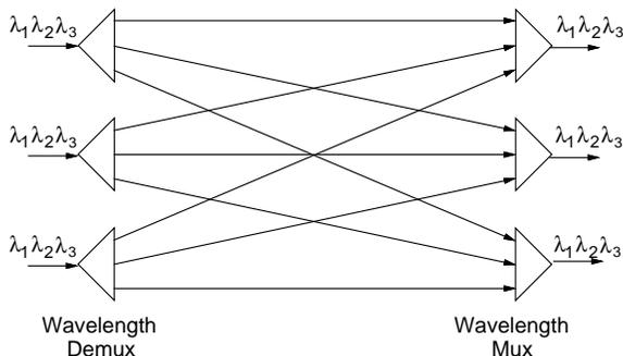
Figure 2: A non-reconfigurable (switchless) wavelength router with 3 ports capable of handling 3 wavelengths per port.
