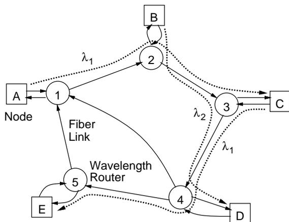
Figure 1: A WDM network consisting of wavelength routers interconnected by point-to-point fiber-optic links. Some of the wavelength routers have nodes attached to them that form the sources and destinations for network traffic.
