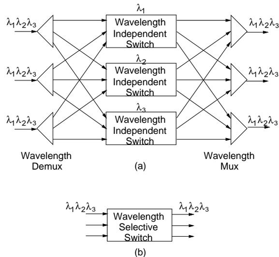
Figure 3: Two types of reconfigurable wavelength switches, each with 3 ports capable of handling 3 wavelengths per port. They can switch each wavelength at its input ports independent of the other wavelengths. The switches can be reconfigured to allow different interconnection patterns. (a) This router uses wavelength-independent switches in combination with passive wavelength demultiplexers and multiplexers. (b) This router uses a wavelength-selective switch.
