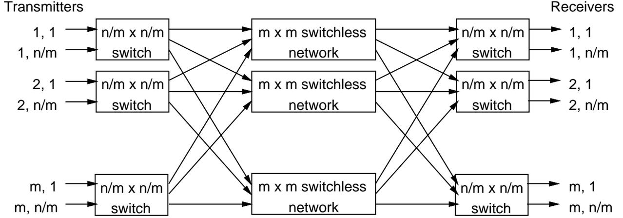
Figure 9: A permutation network using  $w$  wavelengths and  $O(n \log \frac{n}{w})$  wavelength-independent switches.
