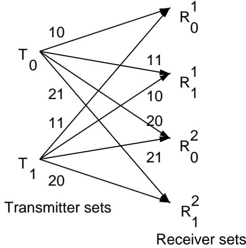
Figure 5: The construction of  $G$  for the case  $b = 2, k = 2$ . The edges are labelled with the wavelengths used for communication.
